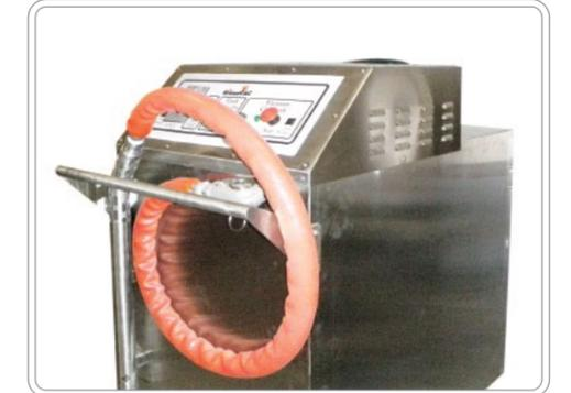
The 75 gallon unit stores about eleven 50lb fryer's worth of oil! The GreaseVAC can extract the oil while it is hot. No time wasted waiting for the oil to cool.
